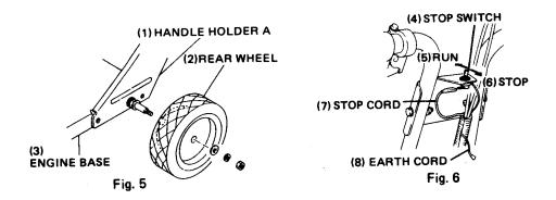
b. To install rear wheels, temporarily remove the nuts, spring washers and washers from the rear axle. Install the rear wheels and secure them with the washers and nuts in the same order. (Fig. 5)
